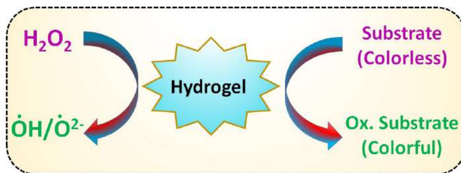
Scheme 1. Fe 3+ -crosslinked hydrogel for peroxidase like catalytic action.
