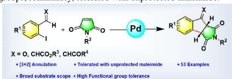
Scheme 1. Palladium catalyzed [3+2] annulation of ortho -Substituted Iodoarenes with Maleimides.
